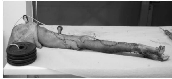
Figure 1. Upper limb cadaveric model before load application
