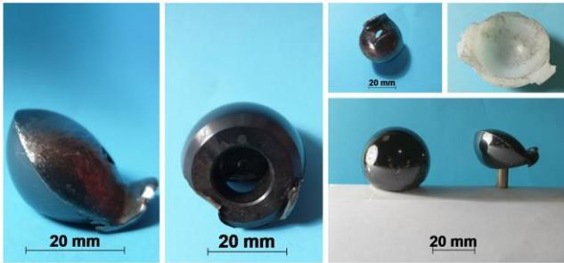
**Figure 3. Pictures of the retrieved polyethylene liner and OxZr head: the breakage of the liner to which its mobilization has followed is clearly visible. The comparison with a new 32mm ball head demonstrates the advanced state of wear and the loss of sphericity.**
