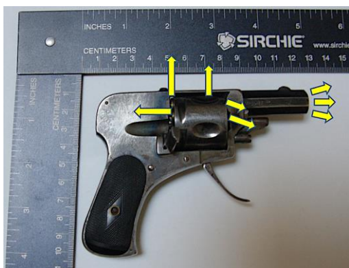
Figure 7. Parts of the weapon from which the gases of firing escape.
