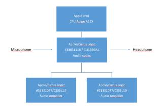
Figure 1. Generation of the signals with the iPad characteristics
