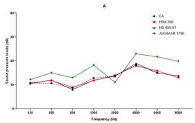
Figure 5. Differences between frequencies detected by different audiometers and related headphones.
